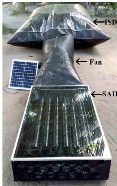
Figure 3. Design of an ISD with integrated SAHs [5].
